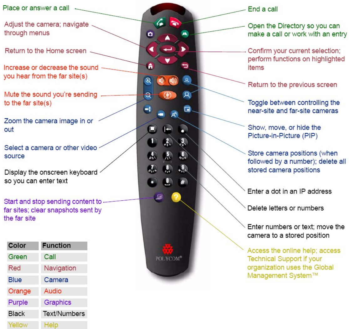
Figure 12: Polycom VSX remote control. Not all versions have separate "Call" and "Hang Up" buttons at the top.
