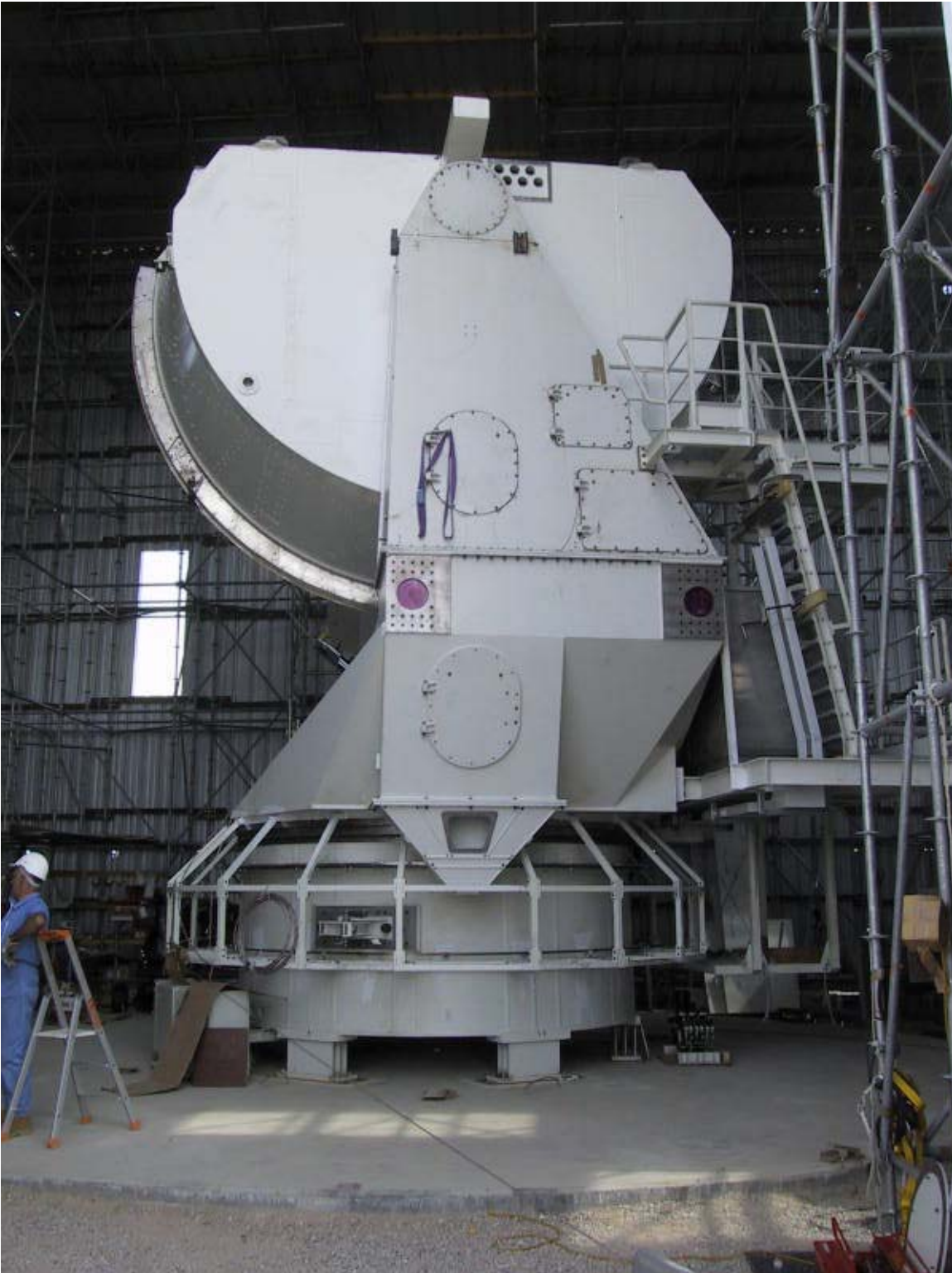
Figure 4. Receiver cabin mounted on antenna pedestal.
