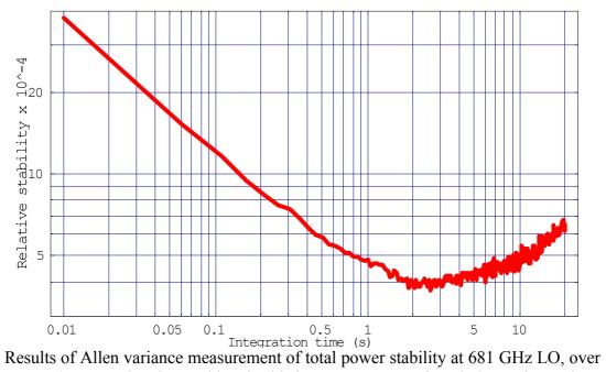
Results of Allen variance measurement of total power stability at 681 GHz LO, over 2 GHz (6-8 GHz band) IF subband. This is a measurement for whole receiver. The source is cold load (77K).
