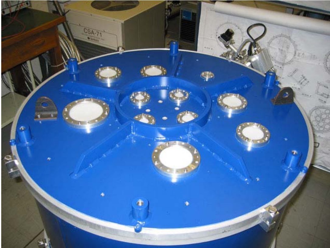
Figure 15. ALMA prototype cryostat fitted with plastic RF windows under test at Rutherford Appleton Laboratory
