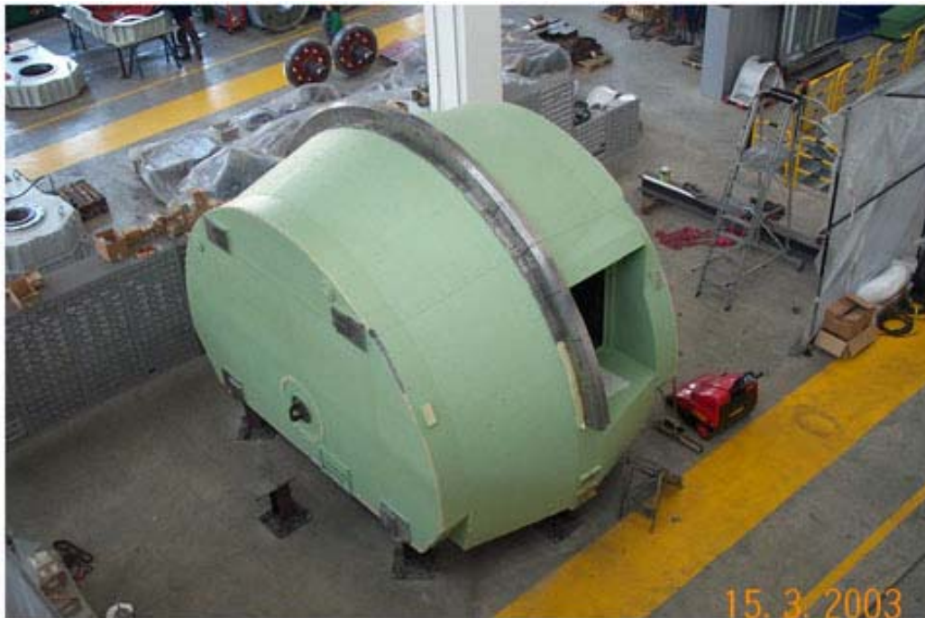
Figure 1. The cabin during painting (primer)
