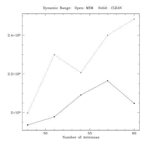
Figure 4: The DR1 dynamic range as a function of number of antennas for the M51 model simulations.
