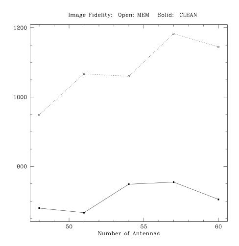
Figure 5: The FID01 dynamic range as a function of number of antennas for the M51 model simulations.
