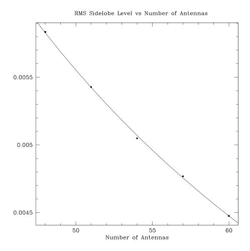
Figure 1: RMS sidelobe level of the 4 hour naturally-weighted PSF as a function of the number of antennas in the array configuration.
