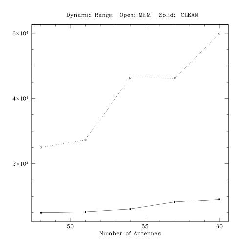
Figure 2: The DR1 dynamic range as a function of number of antennas for the M31 model simulations.
