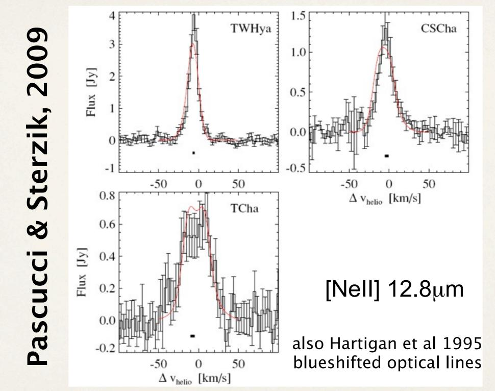
Emission lines formed in the wind will appear blueshifted as the material moves radially towards the observer for specific lines of sight
