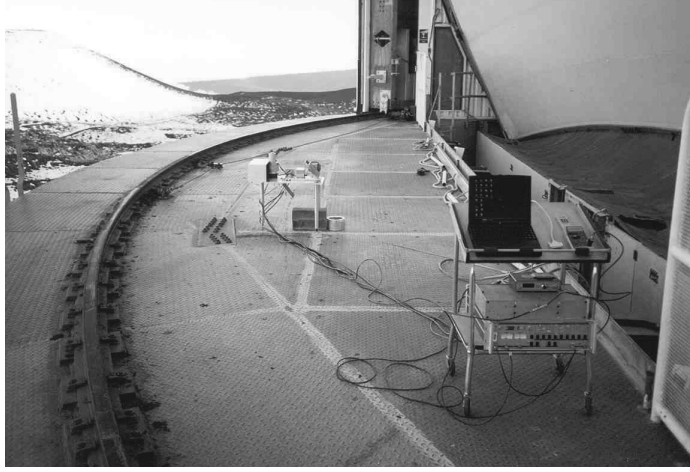
Figure 5: The infrared radiometer, electronics package and laptop control computer on the apron of the JCMT.
