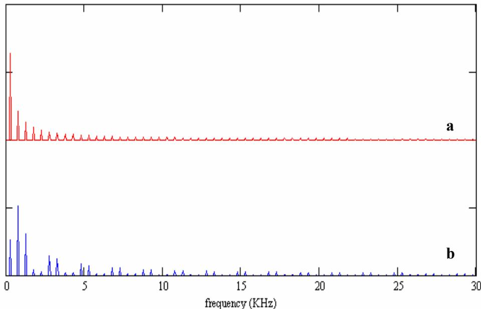
**Figure 2 Voltage amplitudes for the functions (a)  $wal(7,f)$  and (b)  $wal(32,f)$ . The vertical scale is arbitrary and is proportional to the voltage amplitude of the spectrum.**
