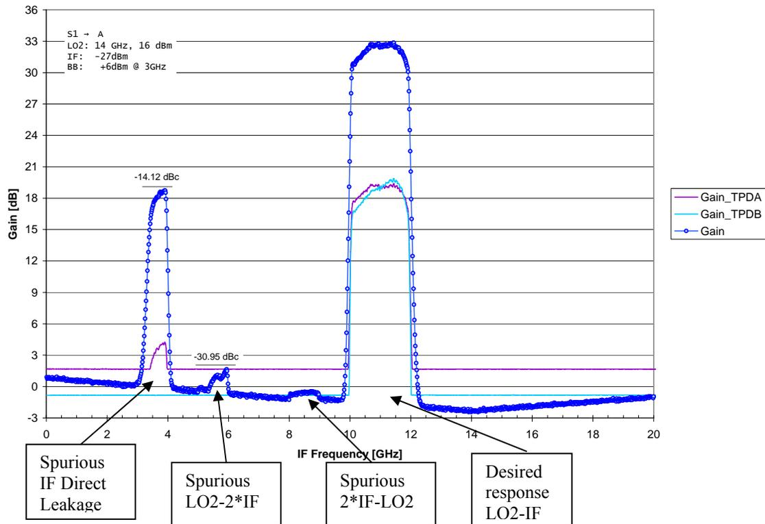
Figure 4 Output power as a function of input frequency for an IFDC with LO2=14.0 GHz
