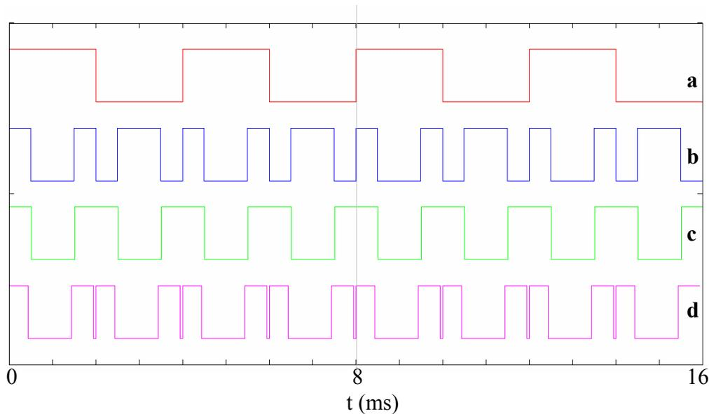
**Figure 1. An example of loss of Walsh function orthogonality due to loss of synchronism. The horizontal time scale is 16 ms, a full period of the slowest Walsh function. All waveforms switch between  $\pm 1$  and are shown vertically displaced to allow comparison. The example waveforms shown are (a)  $WAL(7,t)$ , (b)  $WAL(23,t)$ , (c)  $WAL(7,t)*WAL(23,t)$ , (d)  $WAL(7,t)*WAL(23,t+62.5\mu s)$ .**
