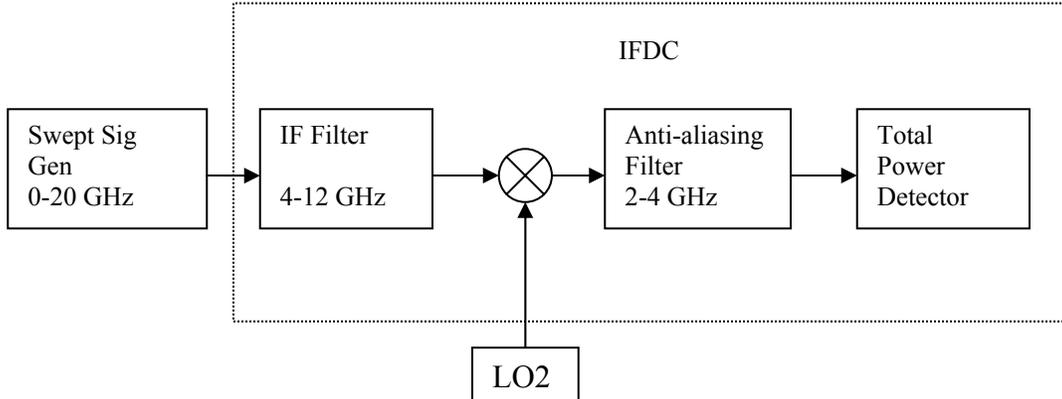
Figure 3 Test setup for measurement of the spurious responses in the IFDC.
