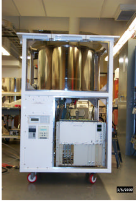
A receiver built especially to evaluate the ALMA prototype antennas, the evaluation receiver, has been constructed at NRAO-Tucson. The receiver contains dual polarization cartridges at 3mm, and single polarization cartridges at 1.3mm. This receiver package will be installed on the Vertex antenna at the ALMA Test Facility site during Autumn 2002.
