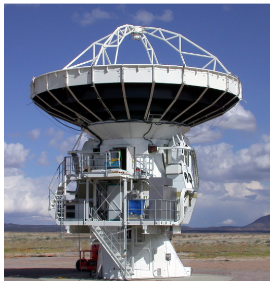
VertexRSI prototype antenna at test facility.
