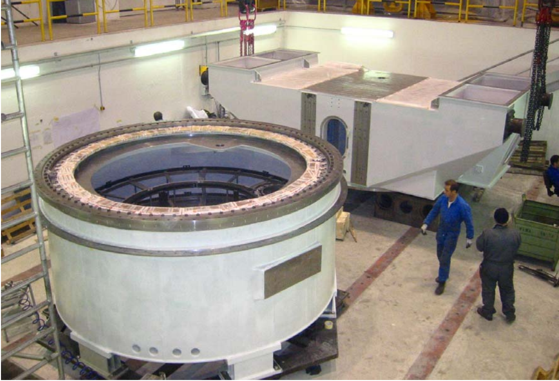
Figure 4. Mount disassembled for packing. Azimuth cable wrap and magnets of the direct drive motor (protected) are mounted inside the base.
