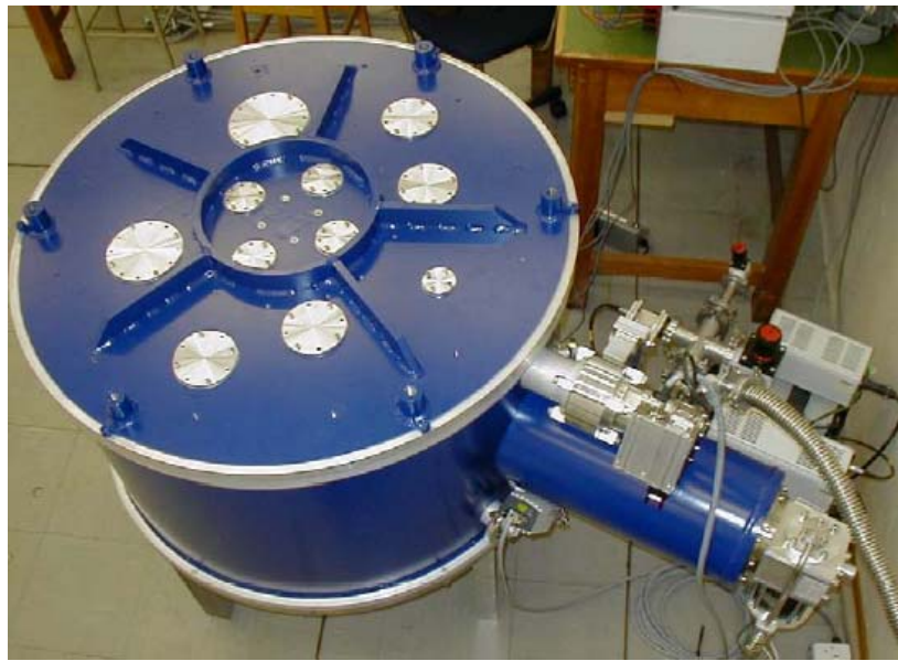
Figure 16. Prototype cryostat under test at Rutherford Appleton Laboratory.
