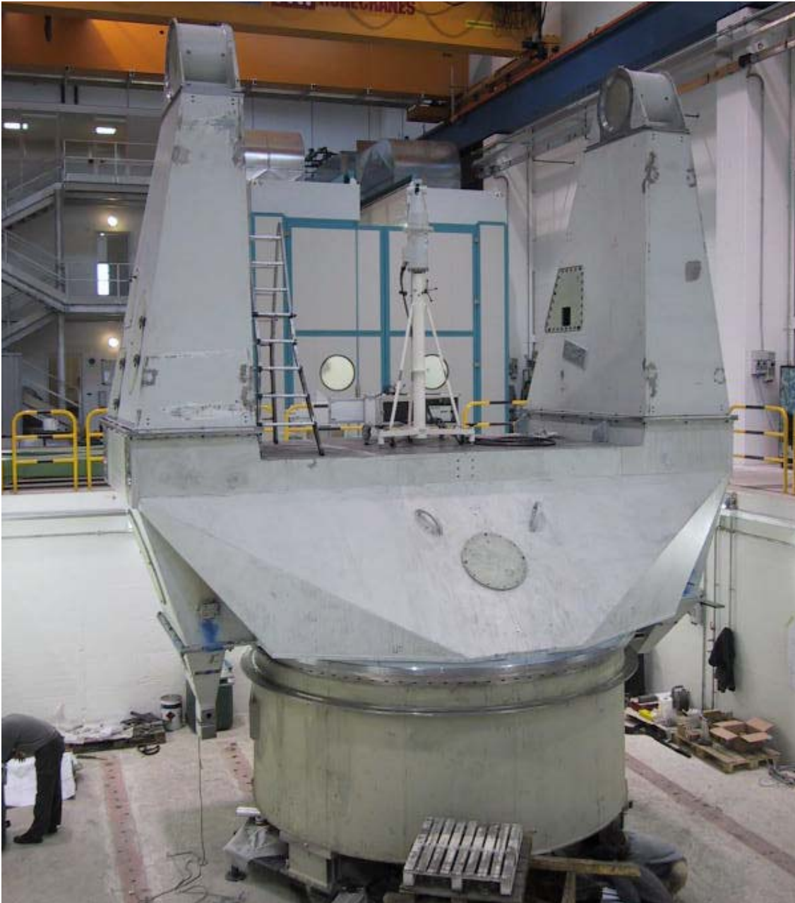
Figure 3. Mount structure during measurements of alignment with laser tracker.
