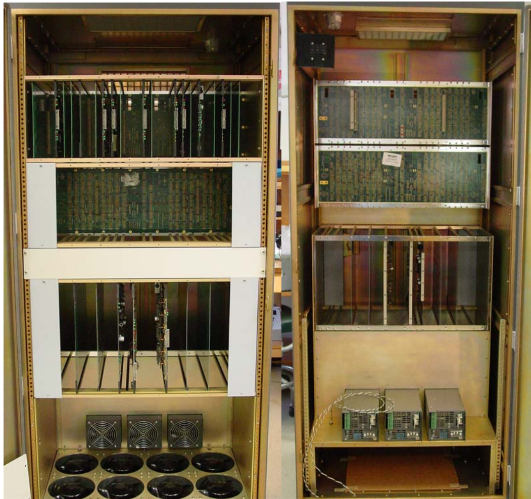
Figure 21. Front (left) and rear of prototype 2-antenna correlator rack showing card cages, cards, backplanes, fans, and power supplies mounted.
