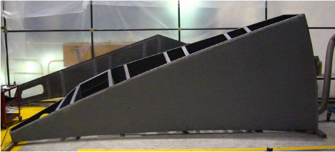
Figure 5. First angular slice of the BUS ready for assembly.
