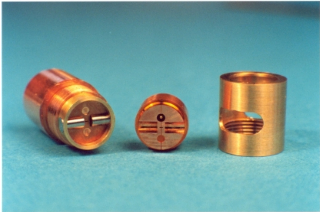
Photograph of newly made waveguide band 9 ALMA mixer. From left to the right: horn with H-field conductors, back piece, fixing nut.
