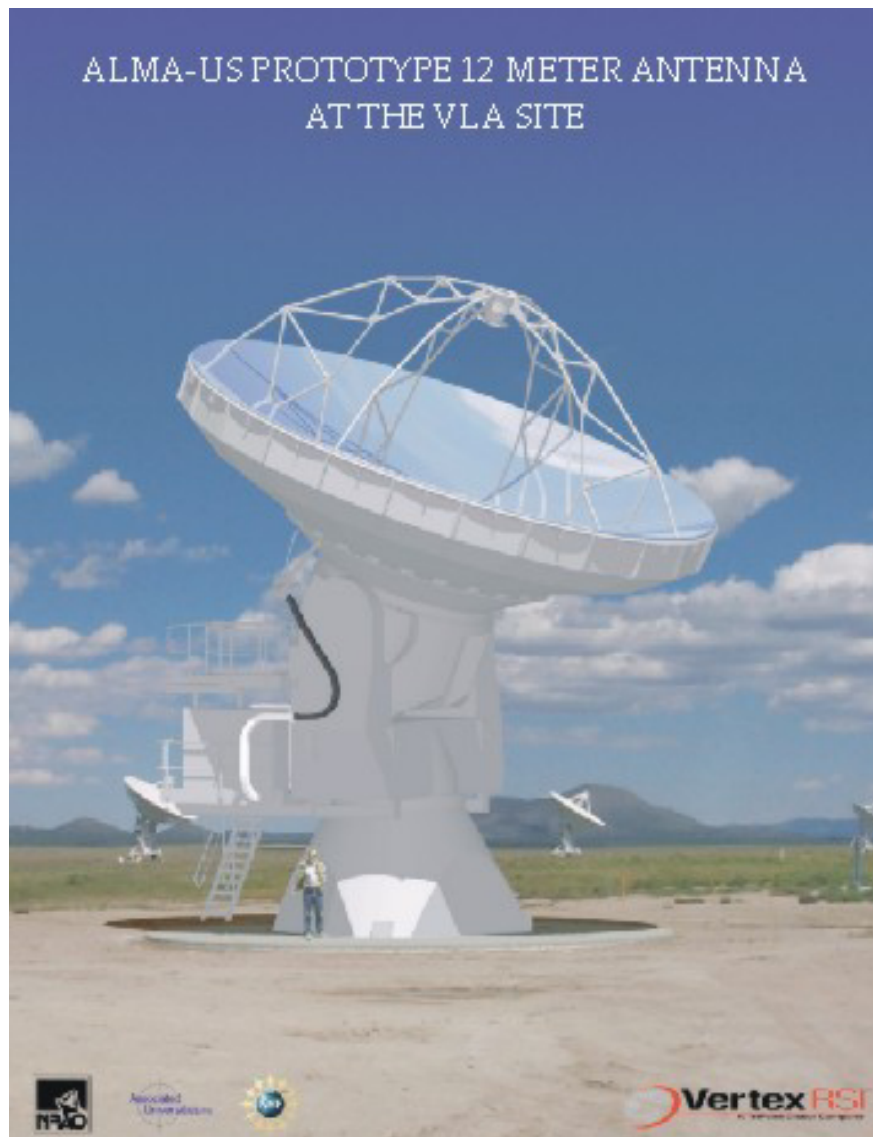
Figure 2. An engineering rendering of the 12 meter diameter prototype antenna that is being fabricated by VertexRSI to the very demanding ALMA specifications. The prototype antenna is under construction at the NRAO Very Large Array site for testing, as shown in this drawing.
