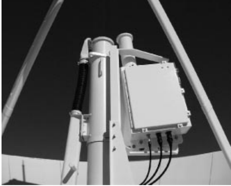
Figure 4. The 22-GHz line radiometer mounted on the 10-m dish of the Usuda tracking station.
