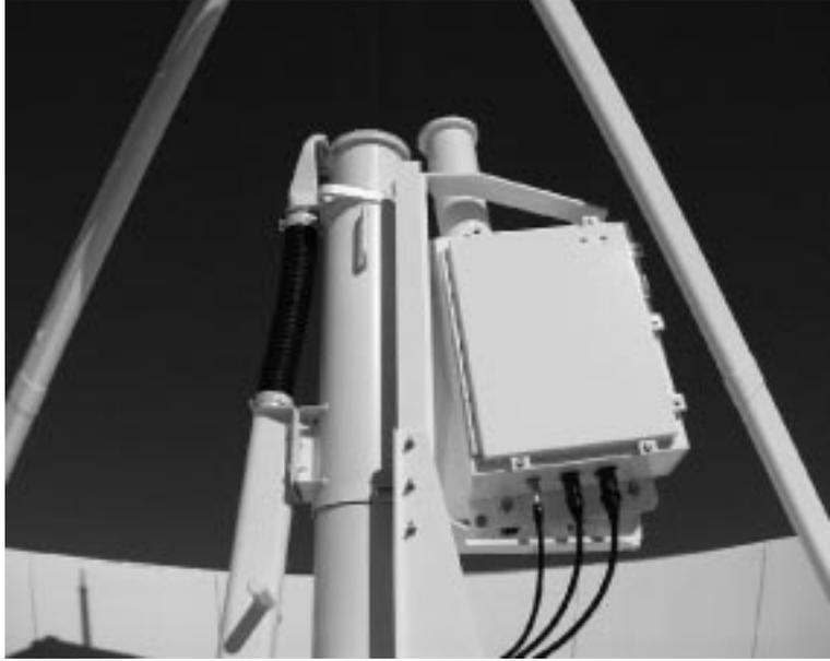
**Figure 4.** The 22-GHz line radiometer mounted on the 10-m dish of the Usuda tracking station.
