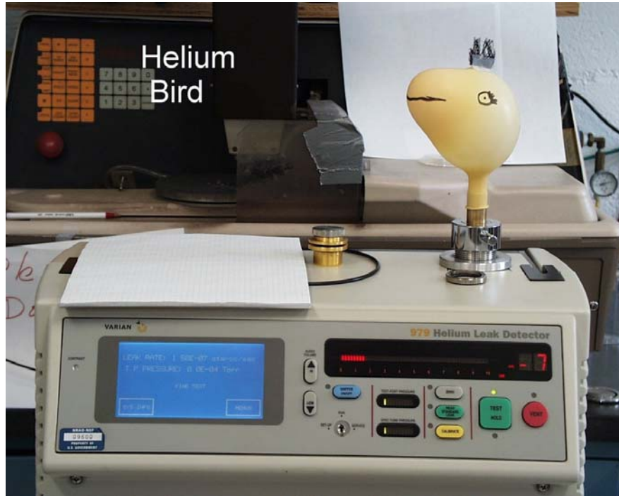
Figure 1: Varian 929 Leak Detector with Balloon Over Device Under Test
