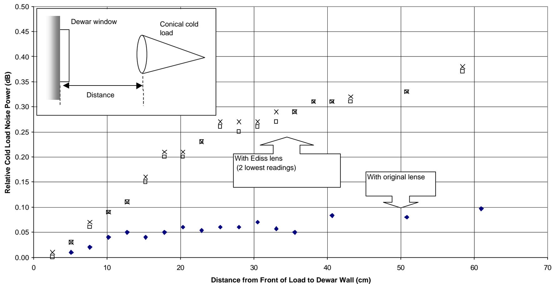
**Figure 4: Cold Load Noise Power vs. Distance 270 GHz**
