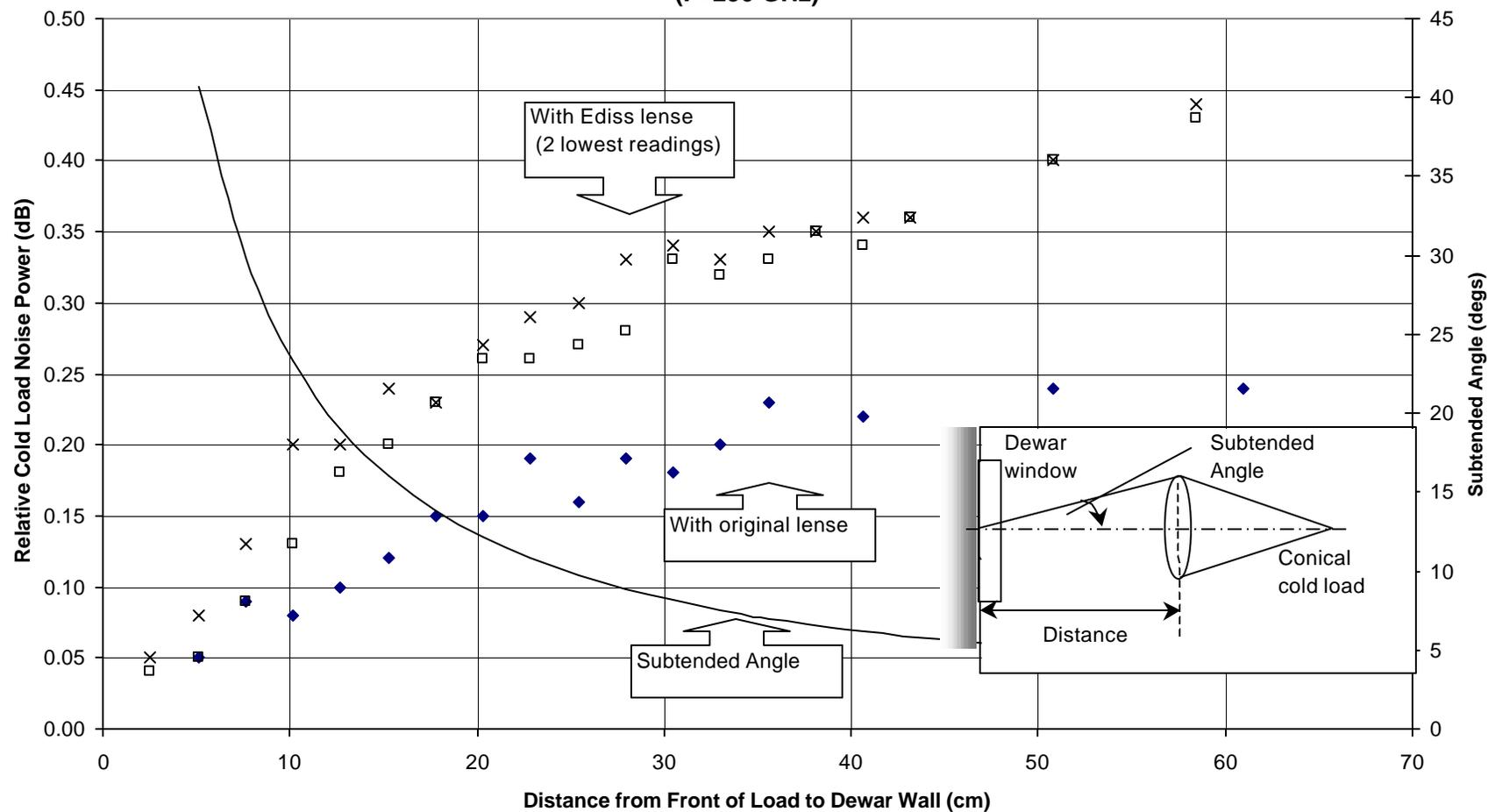
**Figure 3: Cold Load Noise Power vs. Distance 230 GHz**
