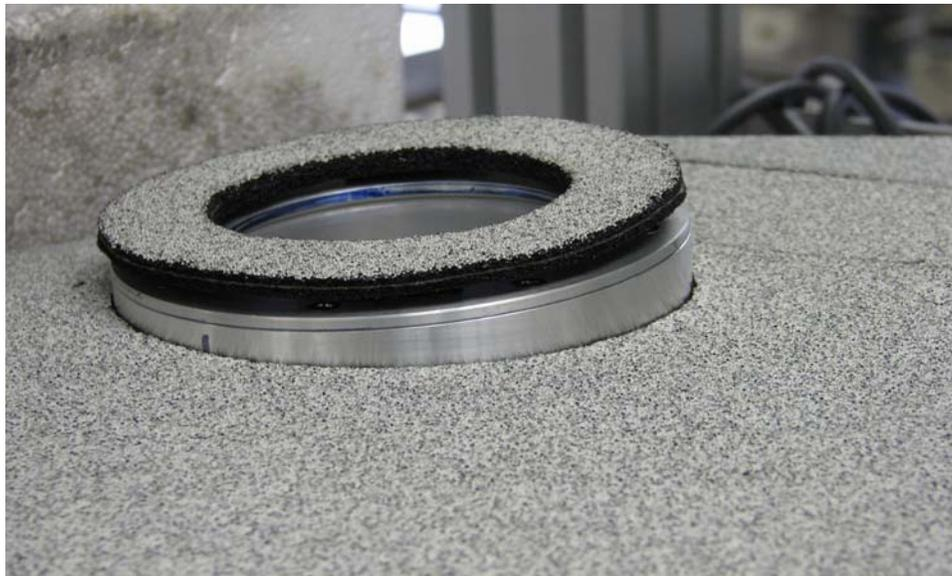
**Figure 4: Vacuum Window Tilted 5 Degrees.**
