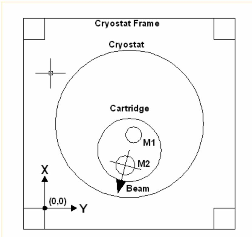
**Figure 8: Orientation of Cartridge in Test Set with Beam Scanner Coordinate Axis Shown.**
