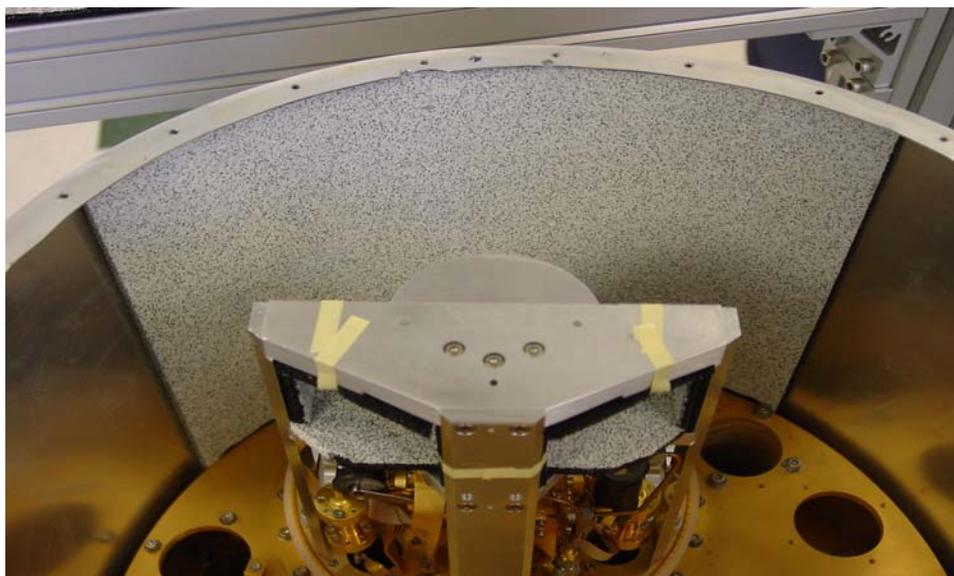
**Figure 6: AN-72 Absorber on Cryostat Wall**
