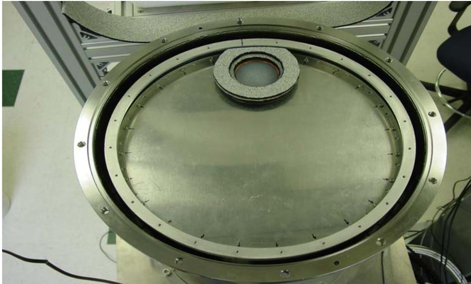
**Figure 7: AN-72 Rings Surrounding IR Filter on Top of 15K Stage**
