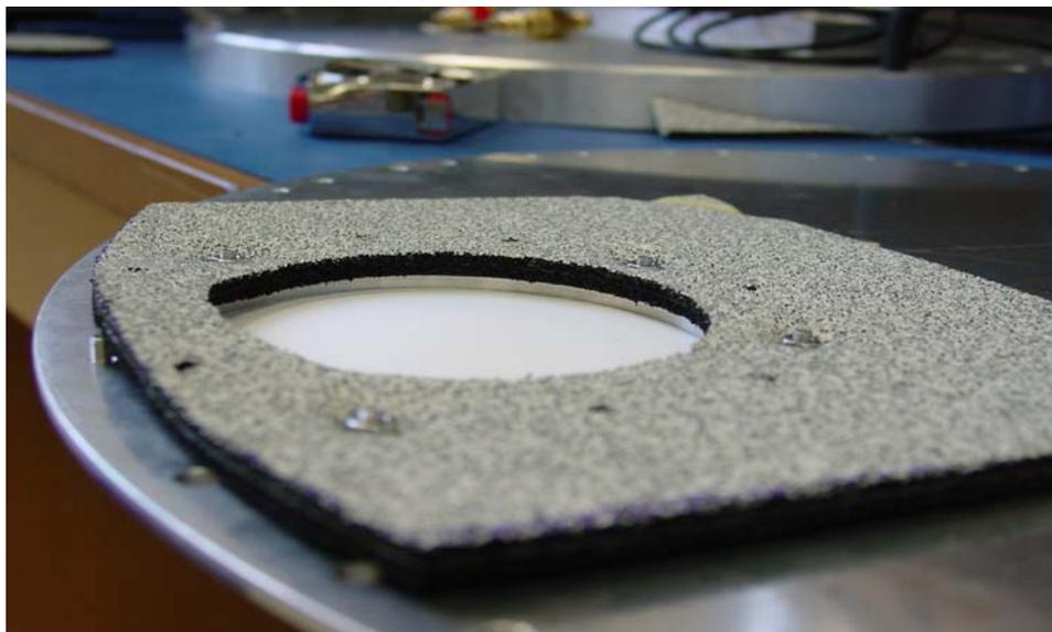
**Figure 5: AN-72 Absorber on Underside of 15K Stage**
