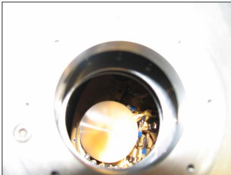
**Figure 5: Band 6 Cartridge in NAOJ Cryostat with IR filters and window removed**
