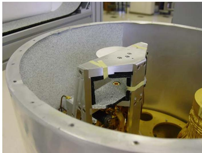
**Figure 9: Absorber *near* horn for patterns with cold cartridge, 2005-02-22**
