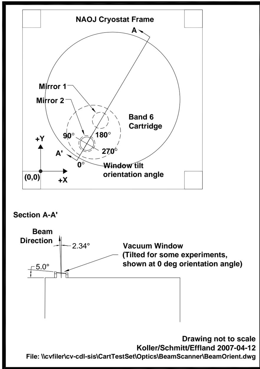
**Figure 3: Coordinate Systems for Pattern Measurements**
