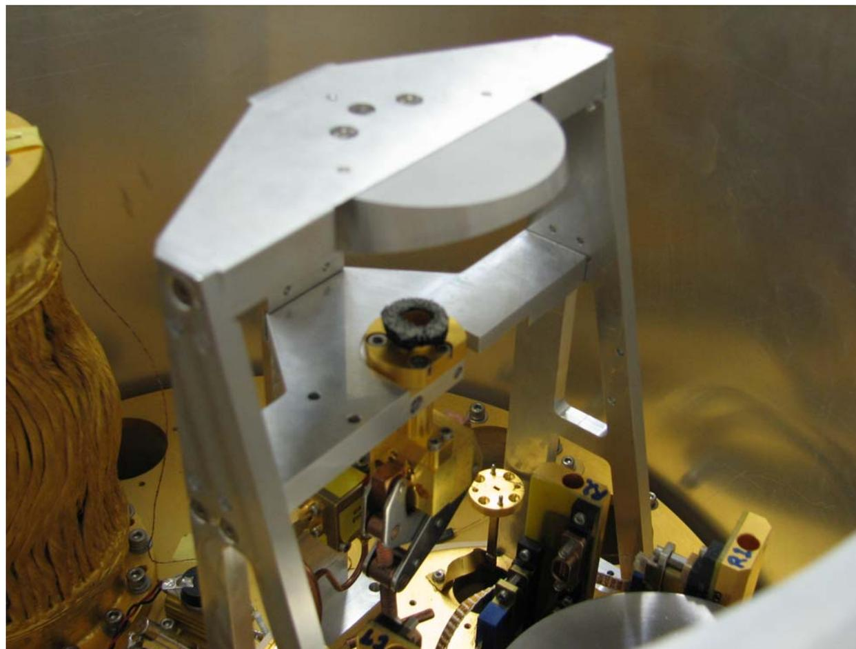
**Figure 8: Room temperature tests of Band 6 Cartridge with AN-72 absorber installed on horn rim**
