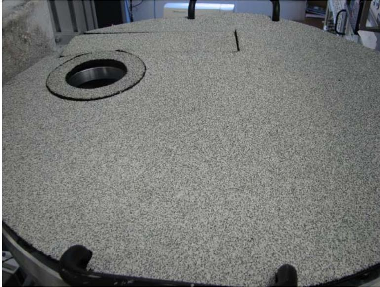
**Figure 4: AN-72 Absorber on top of NAOJ Cryostat with all IR filters and window removed**
