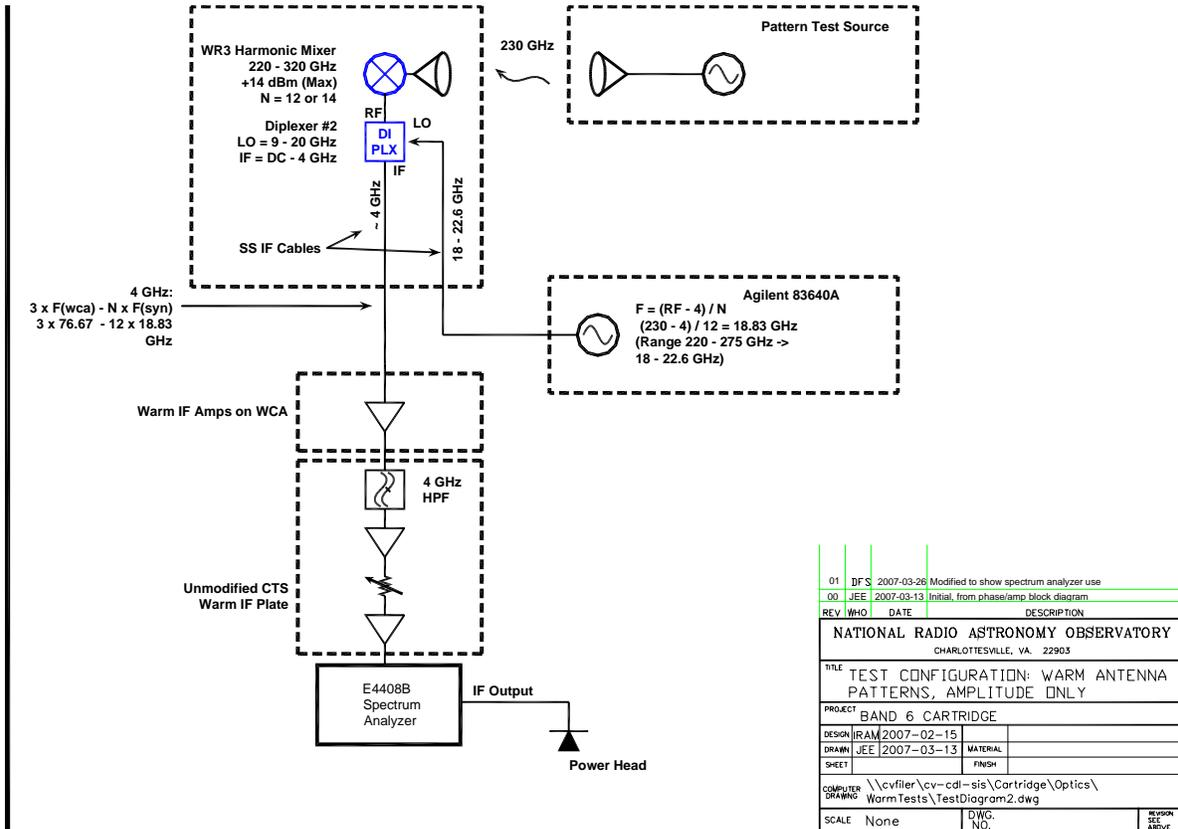
**Figure 2: Room Temperature Mixer Pattern Measurement Test Setup**
