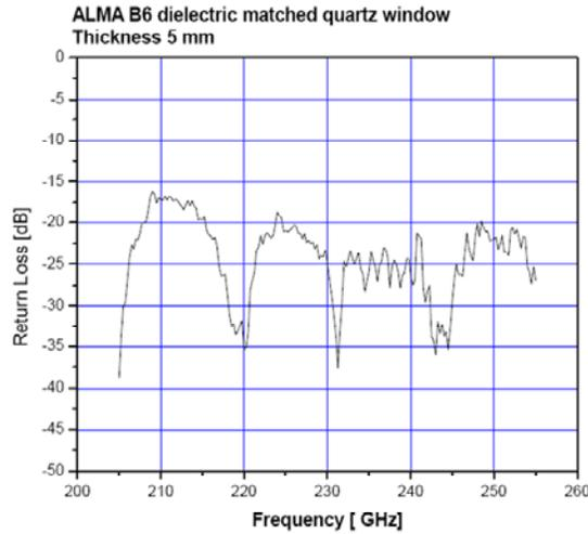
**Figure 1: ALMA Band 6 Vacuum Window Return Loss**
