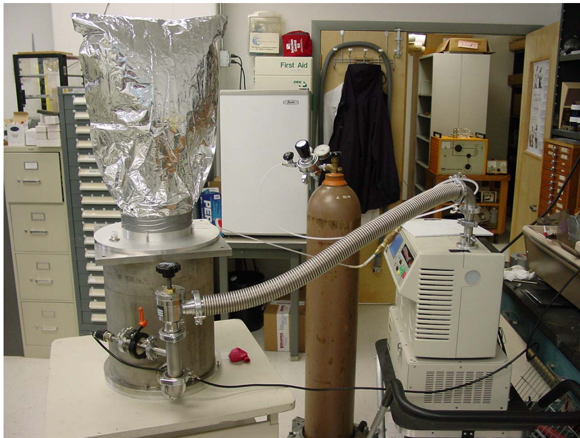
Figure 2: Helium Leak Test Setup, Side View
