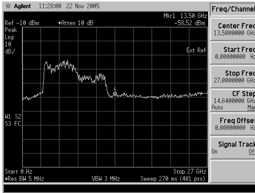
Figure 26: IF Spectrum Measured using HP 35670A
