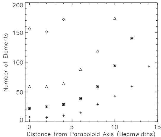
Figure 10: Number of  $0.5\lambda$ -spaced, hexagonal array elements required to collect 80% (crosses), 90% (stars), 95% (triangles), and 98% (diamonds) of the power passing through the focal plane as a function of beam offset.  $F/d = 0.5$ ,  $D = 100\lambda$ .
