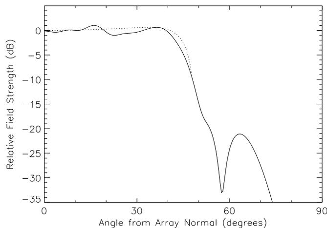
Figure 9: Far-field relative amplitude (solid line) of an  $11\lambda$ -radius, 128-element, hexagonal array on the surface described by Equation 13 using the phase and amplitudes for each element shown in Figure 8. The dotted line is the reflector aperture taper assumed in computing the fields shown in Figure 8.
