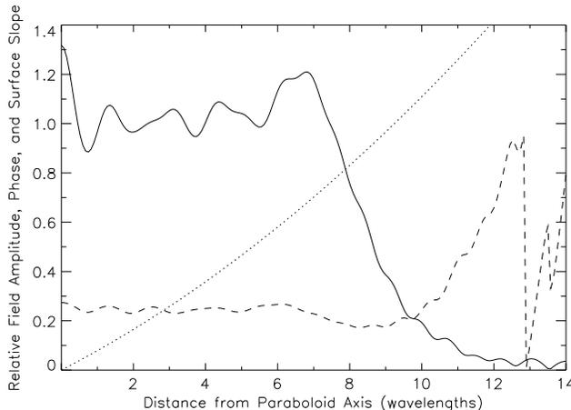
Figure 8: Relative field amplitude (solid line) and phase in wavelengths (dashed line) on the surface described by Equation 13 for a  $100\lambda$ ,  $F/D = 0.56$  paraboloidal reflector. The dotted line shows the slope of the array surface to which the element axes are normal.
