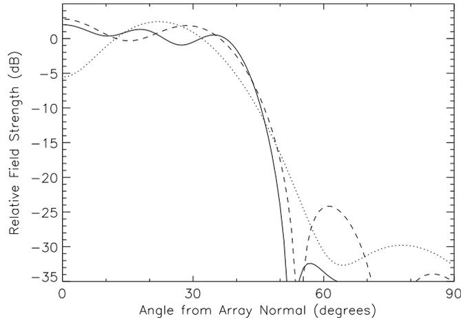
Figure 7: Cross sections of far field patterns of hexagonal arrays of different diameters. The array radii and total numbers of elements are  $4\lambda$ , 139 elements (solid line);  $2\lambda$ , 37 elements (dashed line); and  $1.5\lambda$ , 19 elements (dotted line). In all cases the element spacing is  $0.65\lambda$
