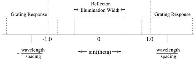
Figure 3. Schematic illustration of grating responses for the illumination of a reflector with  $F/D \approx 1$ . The horizontal axis is  $\sin(\theta)$ , where  $\theta$  is the angle from the array normal.
