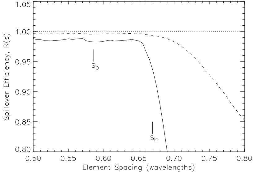
Figure 4. Spillover efficiency vs array element spacing for a two-dimensional hexagonal array designed for  $F/D = 0.56$ .  $S_o$  and  $S_h$  are the angles at which grating responses are expected to enter real space ( $\sin(\theta) < 1$ ) for a rectangular and hexagonal grid array, respectively. The dash line accounts for some grating response suppression from the individual element far field pattern.
