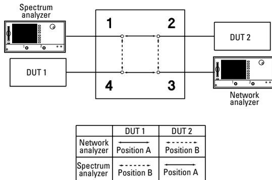
Figure 2. Switching two instruments and two DUTs
