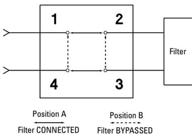
In the signal reverse configuration, a device can be connected across two diagonal ports of the 87222C/D/E transfer switch. This will allow the signal direction through the device to be reversed. See Figure 4.
