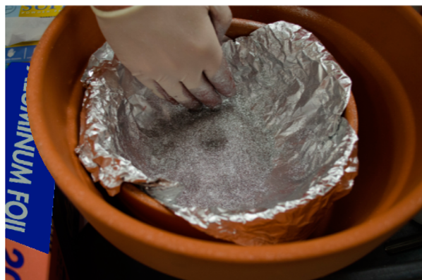
Figure 1. Thermite mixture in aluminum foil containment prepared inside a flower pot. A small divot in the center is formed for containing the ignition powder mixture.
