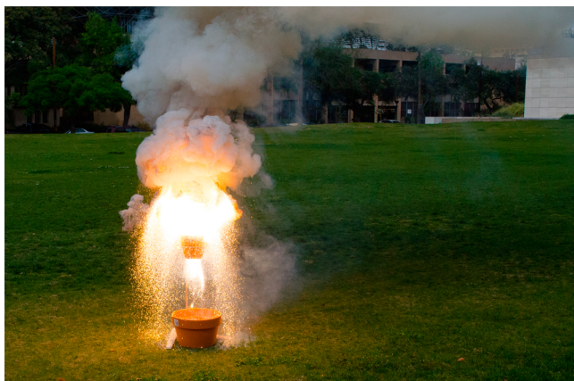
Figure 4. Thermite reaction. The display shown here was prepared with roughly 10 times the amount of thermite as shown in Figures 1 and 3
