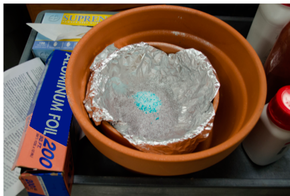
Figure 3. Roman candle ignition mixture added to thermite divot. A second divot is made to accept the H 2 SO 4 .
