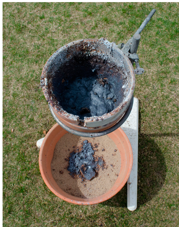
Figure 2. Finished reaction showing the preferred arrangement of a double-layered flower pot suspended above a larger pot filled with sand to catch the molten iron flow.
