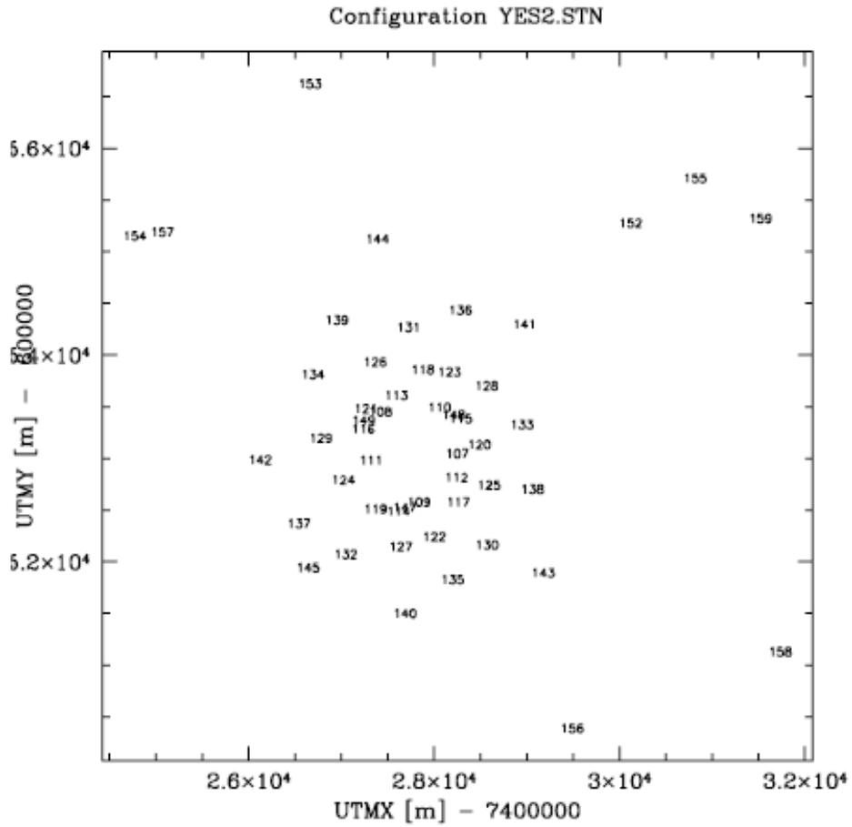
Figure 10 Antenna pad locations for configuration Y2.
