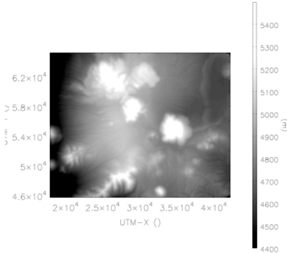
**Figure 1 Digital Elevation model of the Chajnantor site. Note that the coordinates for all FITS files (ie, DEM or MASK) are offset by: UTMX - 600000 m and UTM Y - 7400000 m so that software has sufficient precision - about 1 cm - in single precision floats.**
