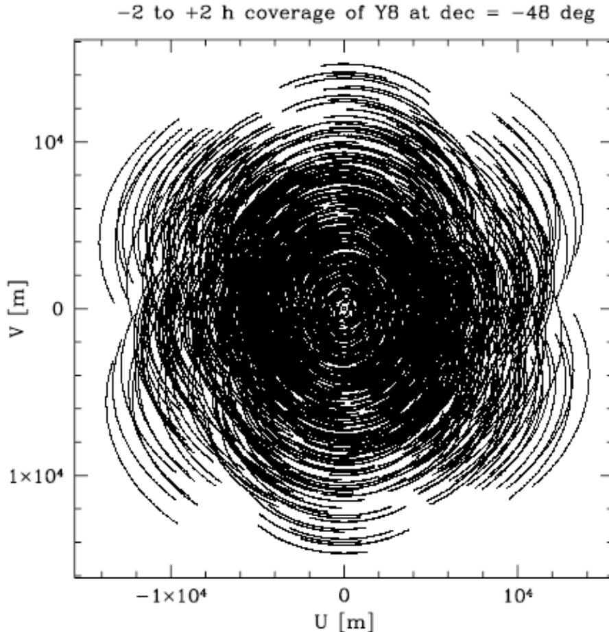
**Figure 7** Plot of the  $(u, v)$  coverage for the Y8 configuration observed at  $\text{dec} = -48^\circ$ , for -2 to +2 hour tracks.
