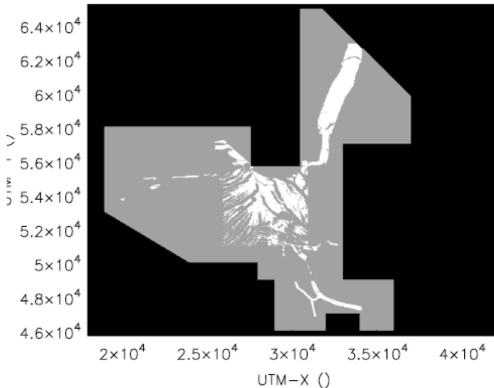
**Figure 4** The Y+ mask with Conway's inner 5x5 km mask inserted, superimposed on the science preserve. Note that the coordinates for all FITS files (ie, DEM or MASK) are offset by: UTMX - 600000 m and UTM Y - 7400000 m so that software has sufficient precision - about 1 cm - in single precision floats.
