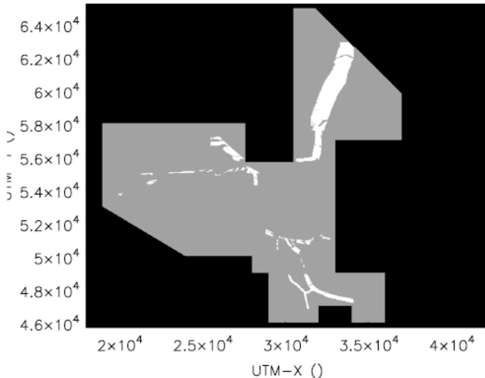
**Figure 3** The final road-based Y+ mask, including gradient, shadowing, viscacha, accessibility, and gas pipeline constraints, superimposed upon the science preserve. Note that the coordinates for all FITS files (ie, DEM or MASK) are offset by: UTMX - 600000 m and UTM Y - 7400000 m so that software has sufficient precision - about 1 cm - in single precision floats.
