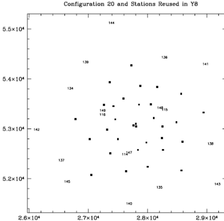
**Figure 5** Conway's outermost configuration #20, with the 18 antennas which are also used in the Y8 configuration numbered.
