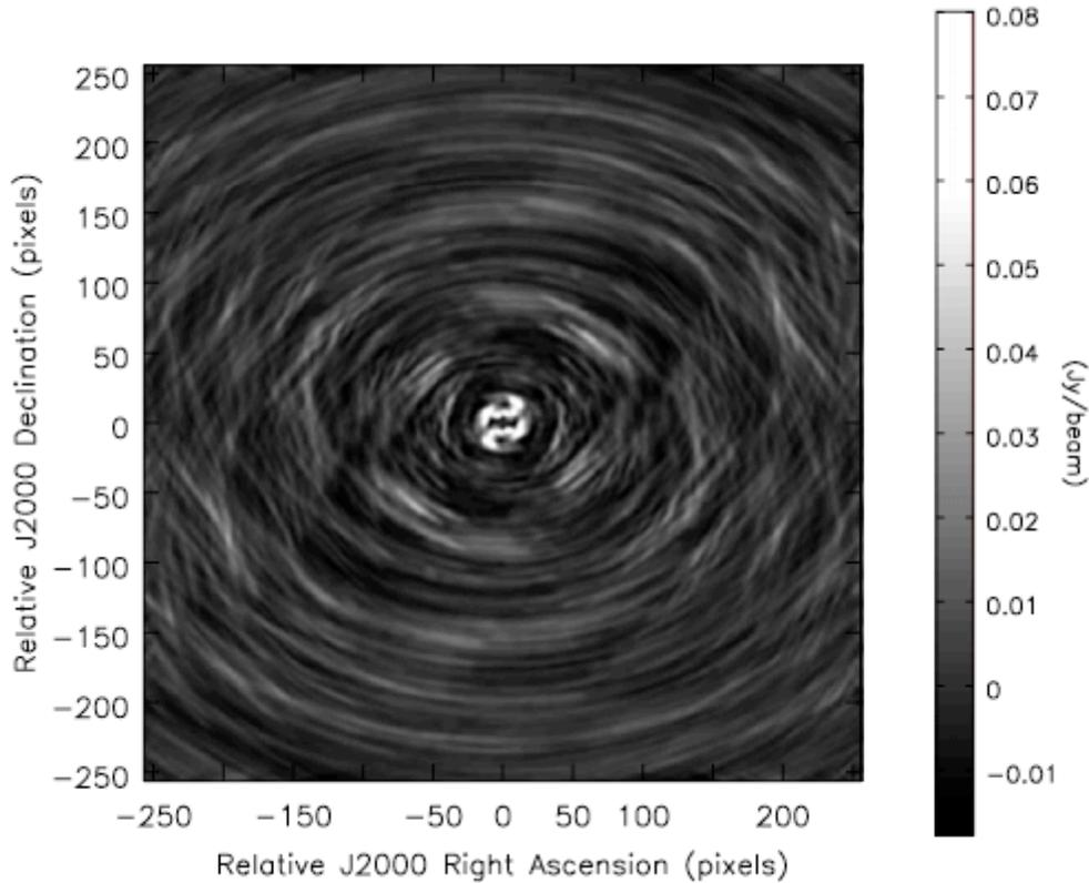
**Figure 8** Plot of the naturally weighted PSF, after removing the best-fit main lobe for Y8 configuration observed at dec = -48°, for -2 to +2 hour tracks.
