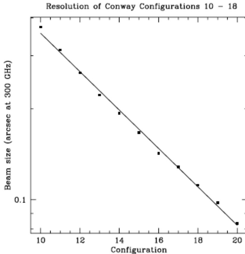
**Figure 6 Naturally-weighted Resolution at 300 GHz of Conway configurations 10-18.**
