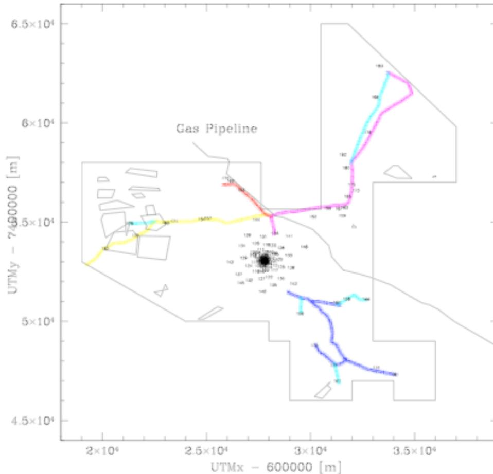
**Figure 2** The science preserve outline, designed roads, gas pipeline, and viscacha colonies (little polygons). Note that the coordinates for all FITS files (ie, DEM or MASK) are offse by: UTMX - 600000 m and UTM Y - 7400000 m so that software has sufficient precision – about 1 cm - in single precision floats.
