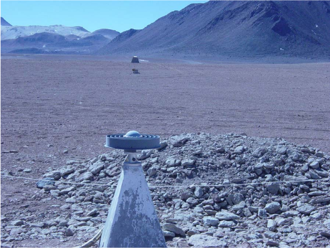
Figure 2: Master0 monument (front), ANM (far back) - The Master0-ANM line defines the local astronomical meridian at this location.
