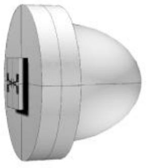
**Figure 5.41 - Quasi-optical SIS mixer configuration**
