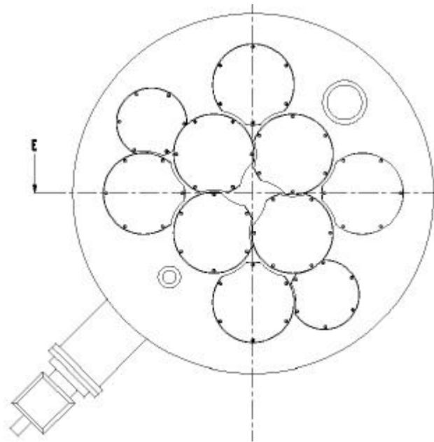
Figure 6-7: : Cartridge location on OVC endplate
