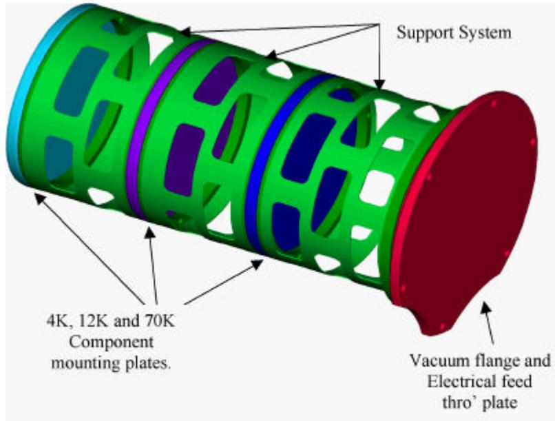
Figure 6-6: : Example of an ALMA receiver cartridge
