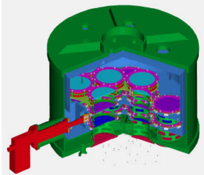
Figure 6-2: Cut-away view of outer vacuum container (OVC)
