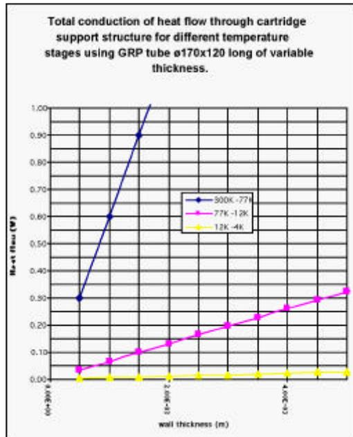
Figure 6-9: Illustration of cartridge support conductive heat flow
