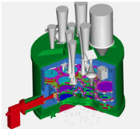
Figure 6-1: ALMA cryogenic system concept showing optics, cartridge and cryocooler arrangement
