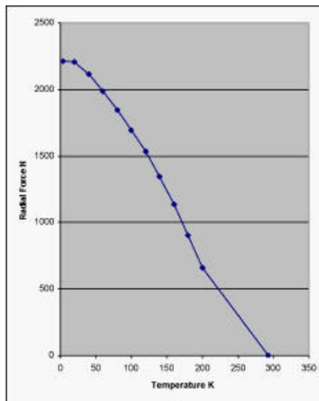
Figure 6-11: : Estimated thermal link clamping forces when cold
