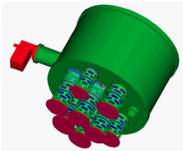
Figure 6-3: Bottom view of cryostat with cartridges extended
