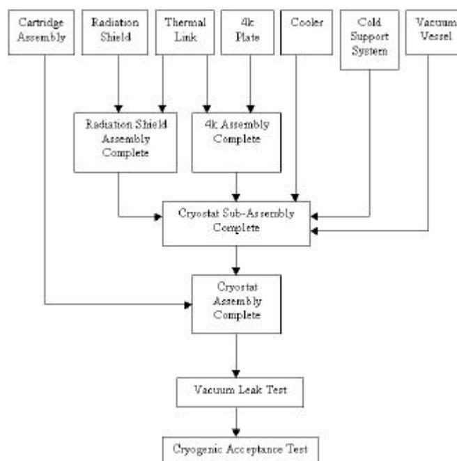
The above flow diagram indicates a suggested methodology for effective production and evaluation of the ALMA cryostat system for the production phase. Completed receiver cartridge assemblies (provided by the receiver groups) would be integrated and tested with the cryogenic system.
