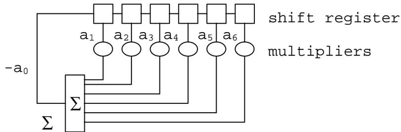
The shift register is shifting from left to right and each element of the shift register must be wide enough to represent all of the levels. If  $q = 3$  then the width must be two bits. If each element of the shift register is viewed as a delay operator then the above loop can be expressed as a polynomial where  $\Delta$  represents a delay.
