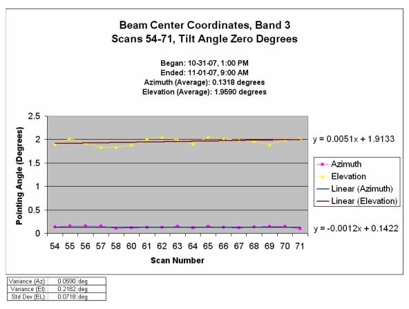
Figure 1 Band 3 beam pointing angles (azimuth and elevation) tilt angle 0 degrees.
