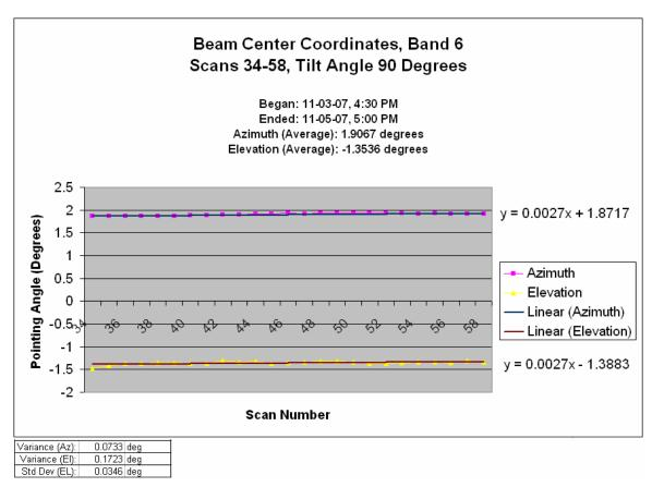
Figure 4 Band 6 beam pointing angles (azimuth and elevation) Tilt angle 90 degrees.
