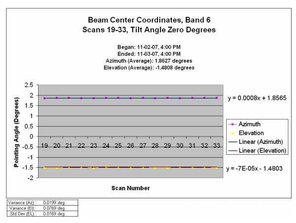
Figure 3 Band 6 beam pointing angles (azimuth and elevation) Tilt angle zero.
