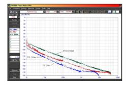
The upper plot shows a real 930 MHz GSM VCO. It shows that the residual noise is low enough to measure "state of the art" new generation VCOs.
